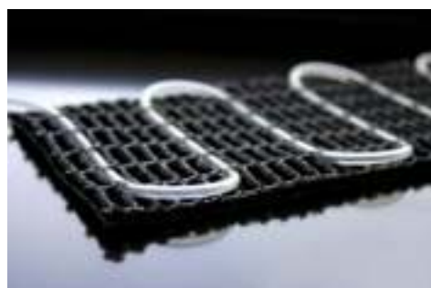
Figure 1 Cooling tubes woven into the textile
