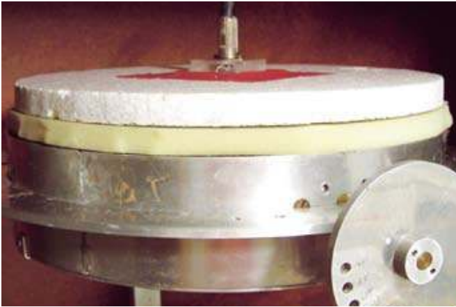
The IFP togmeter. Uppermost in the picture is the measurement plate on the underside of which the temperature sensor T3 is located. The yellow specimen is resting on the reference plate (not visible in the picture) on which the T2 sensor is mounted. Underneath that is the heating plate with sensor T1.
