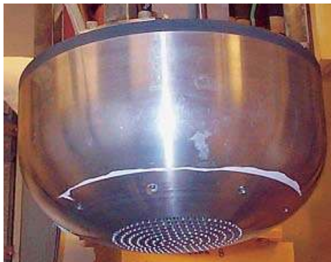
IFP's sweating indentor, underside
