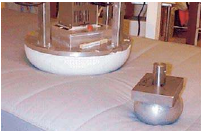
Large and small indenter for the measurement of pressure distribution.
