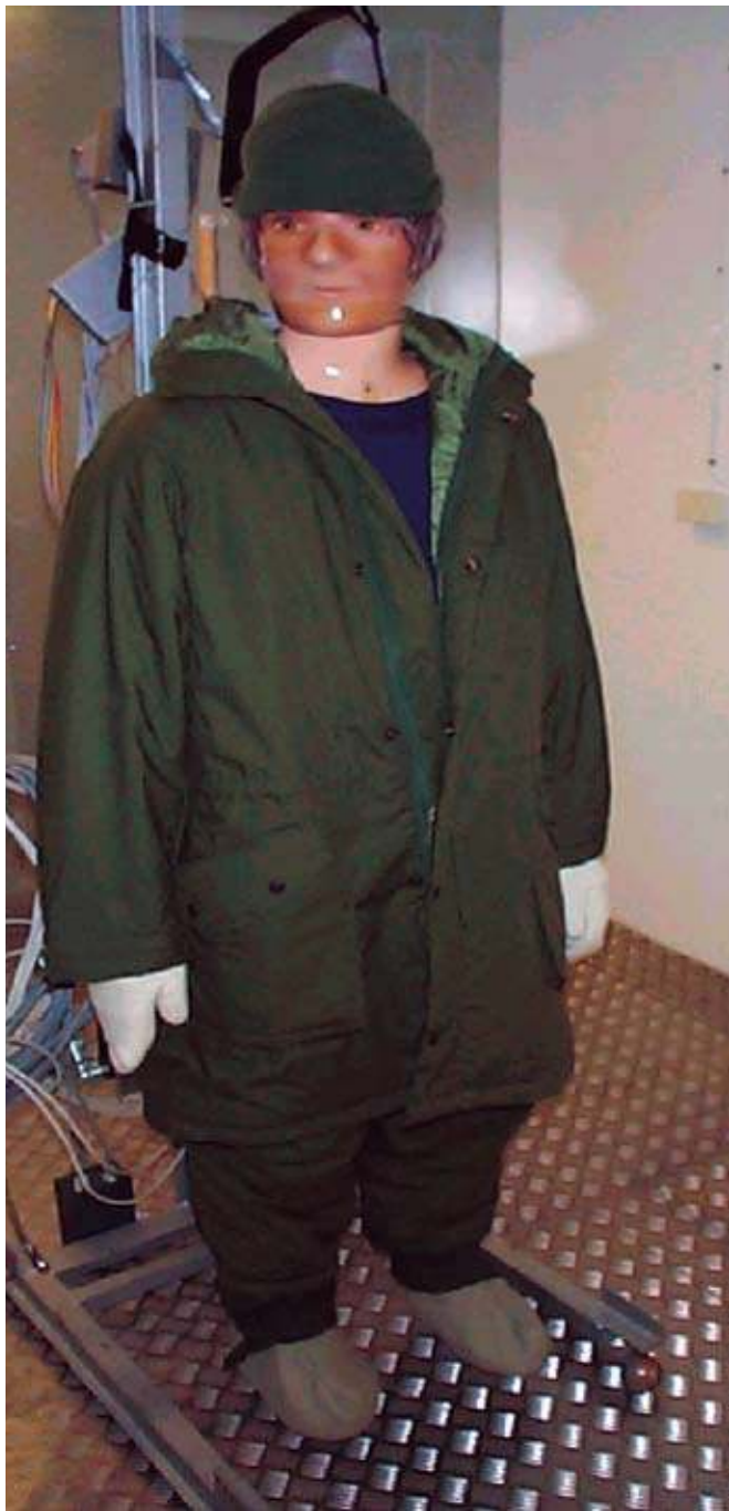
Standing dummy. Testing of winter clothing.
