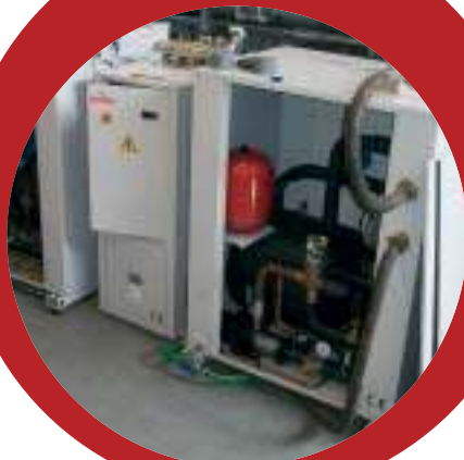
Prototypes of propane heat pump ready for testing.
