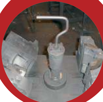
A permanent mould for manufacturing aluminium castings.
