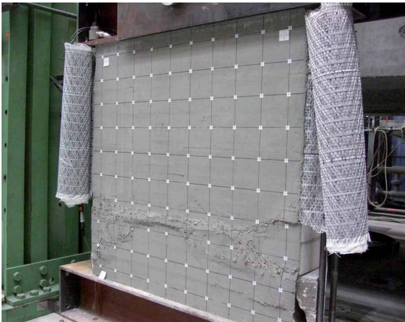
Figura 5. Test di tappezzeria composita antisismica condotto presso il Karlsruhe Institute of Technology (KIT, Germany) Figure 5. Testing of seismic wallpaper composite carried out at the Karlsruhe Institute of Technology (KIT, Germany)
