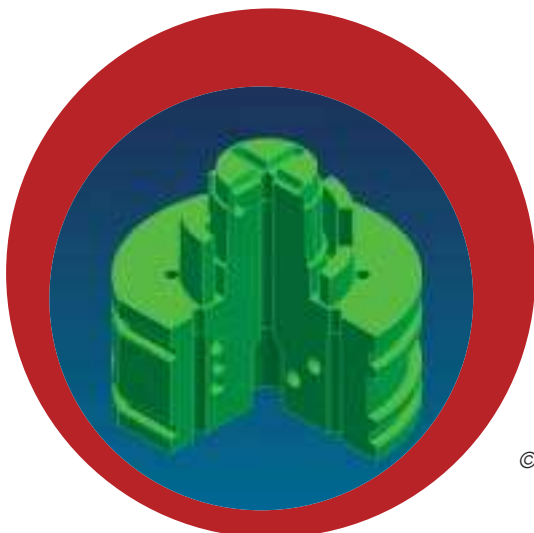
Example of CAD-file with internal conformal cooling channel configuration; separate channel shown in extraction.
