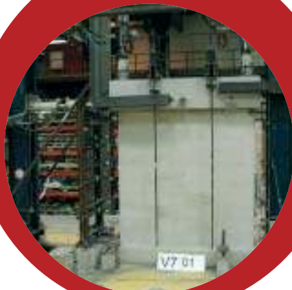
Testing the strength of masonry walls.
